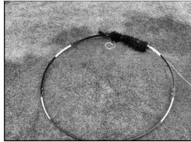
Once the circular frame is complete, pull the tube net with the white bungee cord around the circle. Insert the cut end of the bungee cord drawstring through the loop on the other end and pull to tighten. Cut the excess cord off and tie the two ends of the tube net together with the black tag lines on each end. Try to keep the seam rope on the outer edge of the frame for uniformity.
