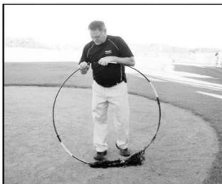
Assemble the circular frame (ring) first... Match the color coded ends and insert the pieces into the coupler. Bolt them together by using the 1/4" bolts and lock nuts provided. **Make sure the bungee cord is inside the tube net before sliding the tube net onto the frame. This must be done before the frame is completely assembled.**
